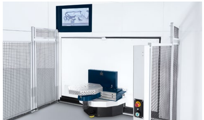
With the additional status monitor, you can also keep an eye on the process remotely.
