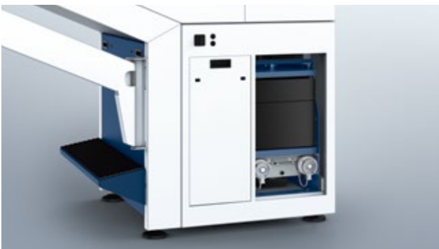
The integrated extractor protects staff from smoke and particles.
