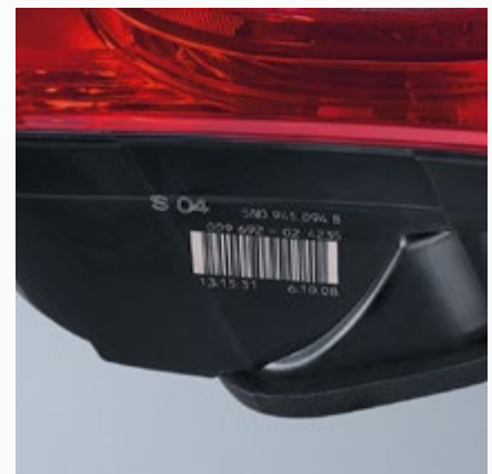
By foam marking: Barcodes and marking rear car lights with free text.
