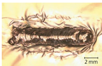
Welding of battery foil stacks consisting of 100 copper foils with TruDisk 2021.
